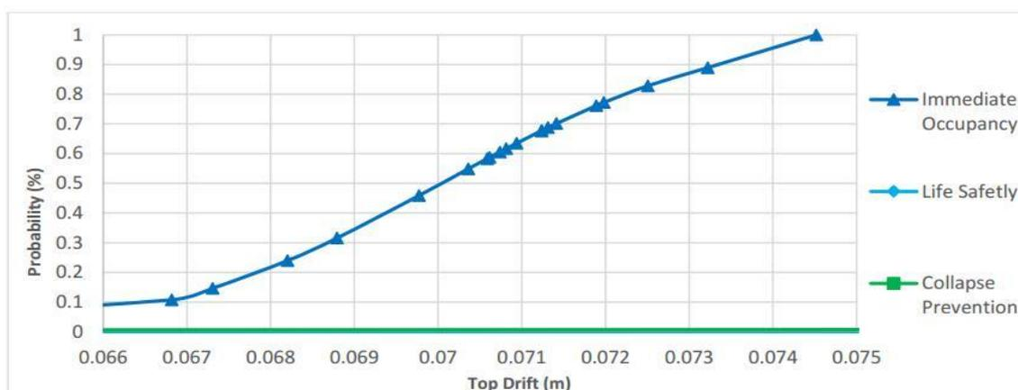
**Figure 6. the normal distribution probabilistic fragility curves regarding top drift (m) RC building Frame.**
