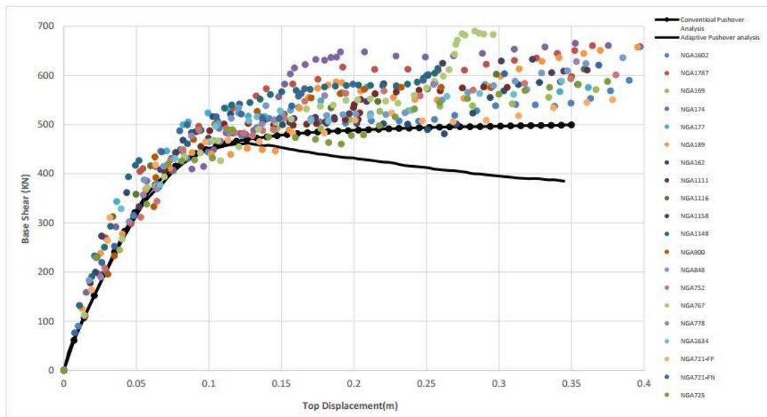
**Figure 8. Capacity curves of RC Building frame, determined by performing conventional pushover and DAP, compared against IDA envelopes**
