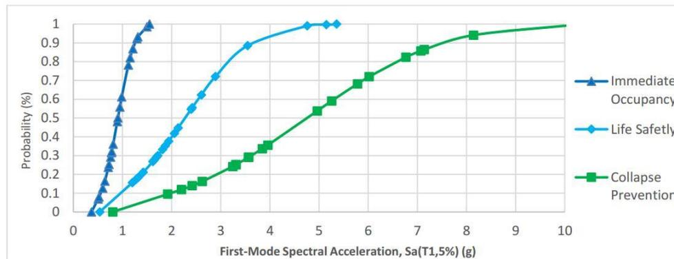
**Figure 5. The normal distribution probabilistic fragility curves regarding PGA RC building Frame.**
