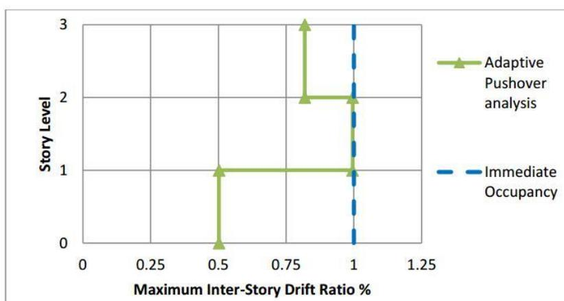
Figure 7. Inter-story drift profiles of RC Building Frame
