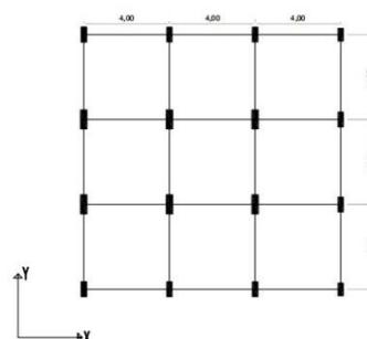
Figure 3. structure and story RC structure is 12 m by 12 m in plan
