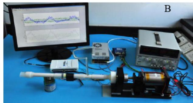
**Figure 1:** Scheme of the FOT device hardware structure (A) and the real prototype of the FOT device (B).
