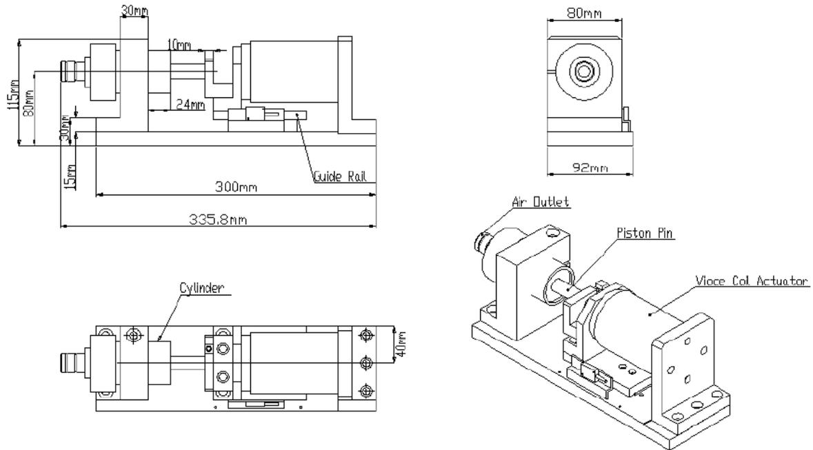
**Figure 2:** Diagram of the voice coil actuator.
